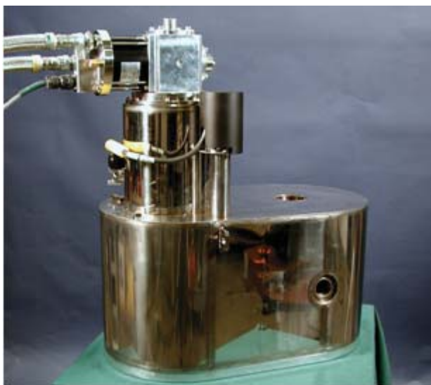
Radial access RTB magnet system
